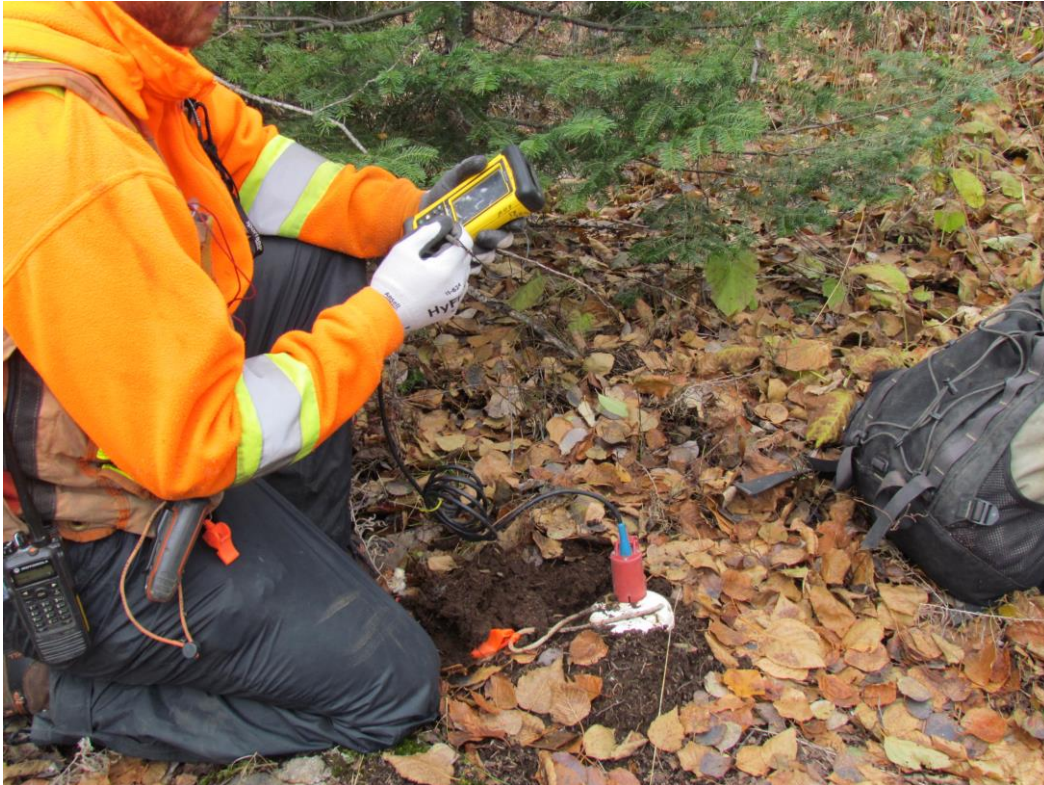
Figure 3: Node placed in a small hole in the ground at Marathon test site.
